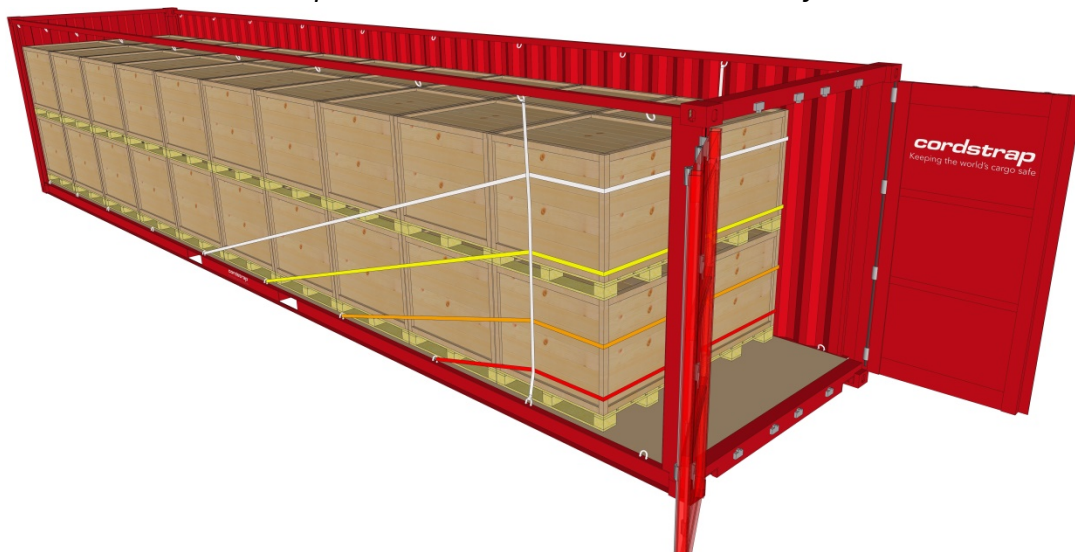
Cordstrap AnchorLash® 105.4 solution in a 40 ft CTU
