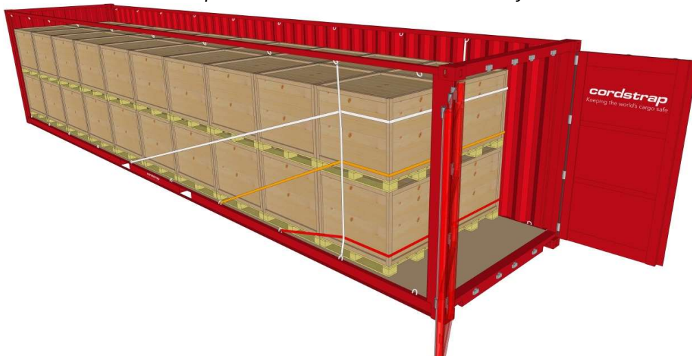
Cordstrap AnchorLash® 150.3 solution in a 40ft CTU
