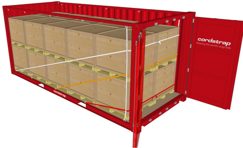
Cordstrap AnchorLash® 150.3 solution in a 20ft CTU
