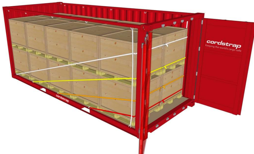
Cordstrap AnchorLash® 105.4 solution in a 20ft CTU
