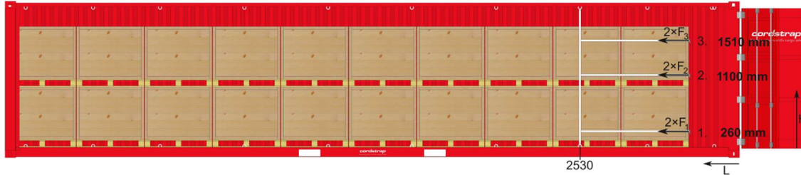
Cordstrap QuickLash® 105.3 solution in 40ft CTU
