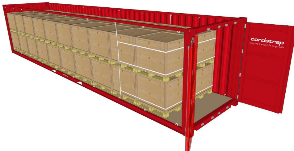
Cordstrap QuickLash® 105.3 solution in a 40ft CTU
