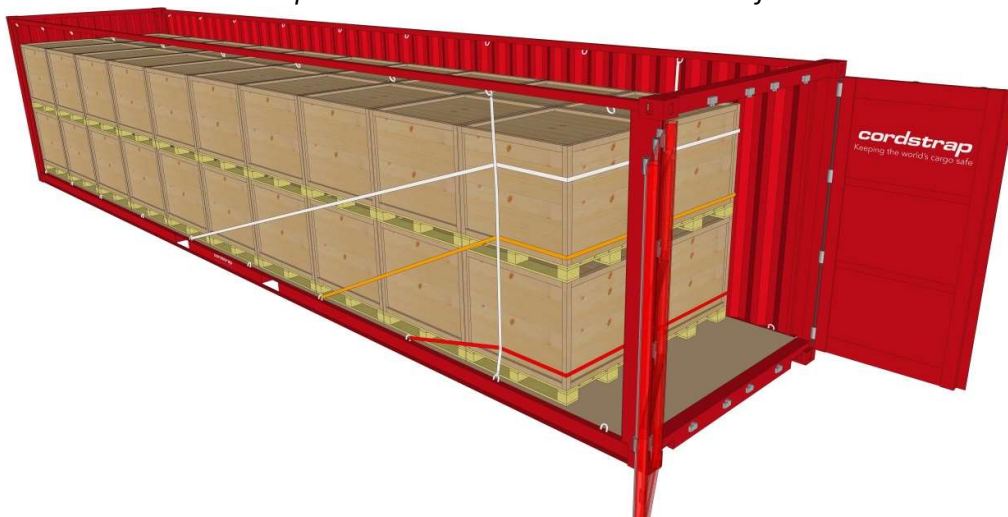
Cordstrap AnchorLash® 150.3 solution in a 40 ft CTU
