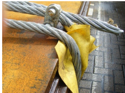
Figure 7.11 Poor edge protection
