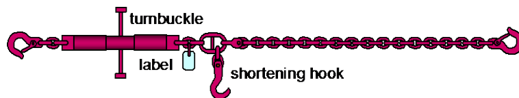
Figure 7.18 Standard chain lashing with shortening hook
