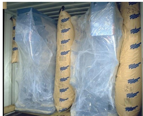
Figure 7.10 Irregular shaped packages blocked with dunnage bags
