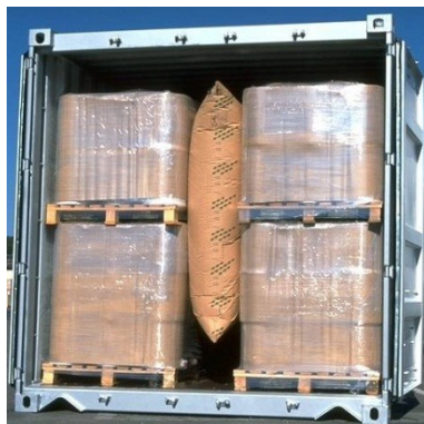
Figure 7.9 Gap filled with a central dunnage bag
