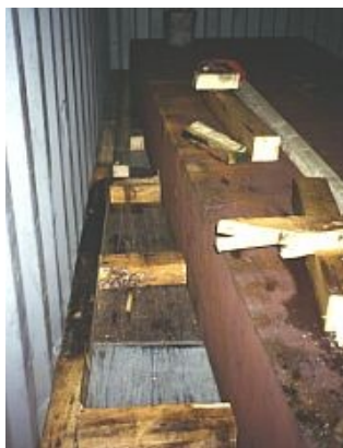
Figure 7.45 Transverse blocking of steel slab
