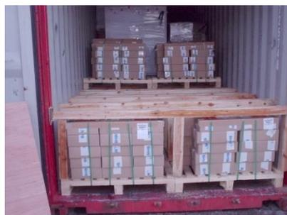
Figure 7.2 Timber temporary floor
