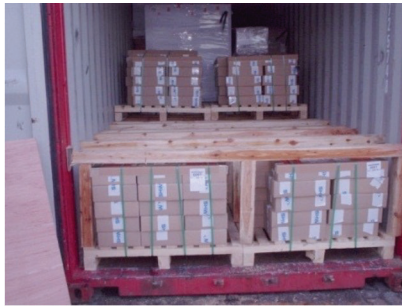
Figure 7.2 Timber temporary floor
