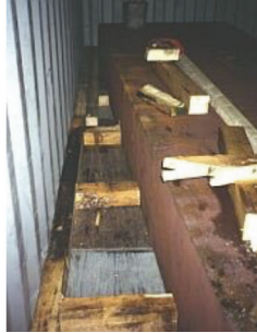
Figure 7.45 Transverse blocking of steel slab
