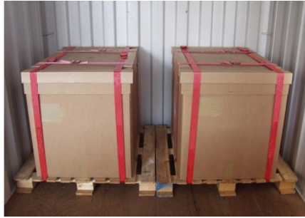
Figure 7.8 Cargo firmly secured to pallets by textile lashings
