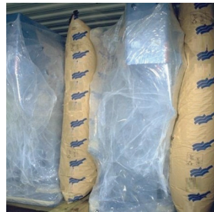
Figure 7.10 Irregular shaped packages blocked with dunnage bags
