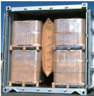
Figure 7.9 Gap filled with a central dunnage bag
