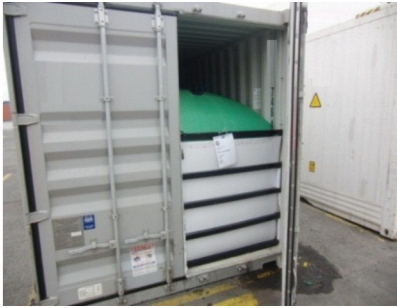
Figure 7.51 Container fitted with flexitank
